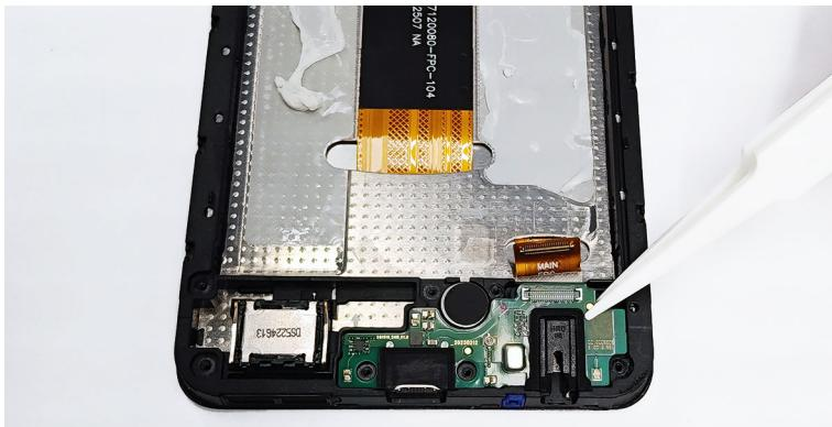
7. Remove the speaker and the vibrator from the front cover.
