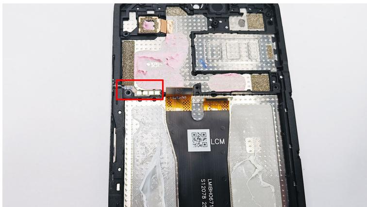
13. Remove the side key FPC from the exterior of the front cover.
