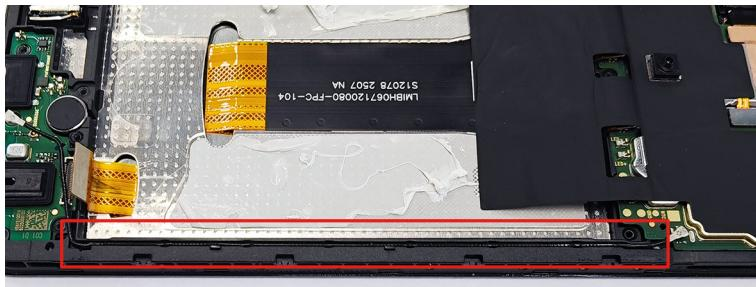
4. Remove the graphite sheet from the mainboard.
