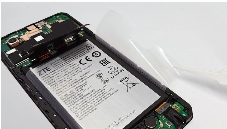
9. Lift up the film to separate the battery from the front cover.
