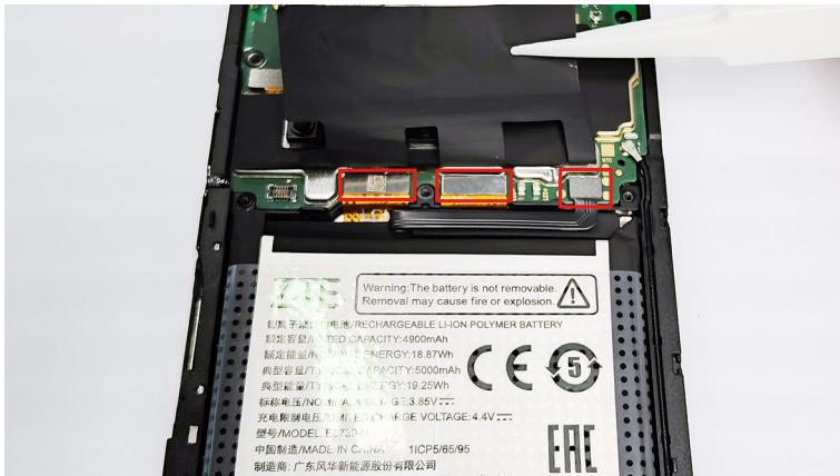
8. Remove the film from the top surface of the battery.
